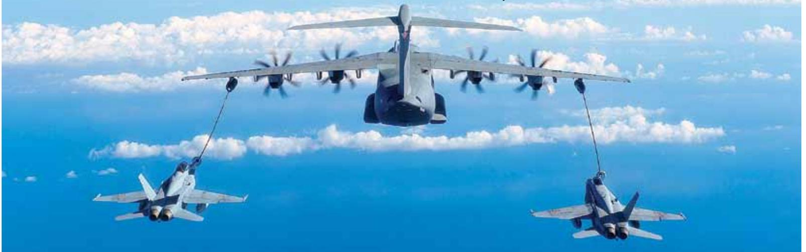
The Airbus A400M new generation airlifter has further proved its credentials as a tanker by successfully demonstrating simultaneous air-to-air refuelling of two F/A-18 fighters. In the course of four flights, the A400M performed 74 contacts and dispensed 27.2 tonnes of fuel to the Spanish Air Force aircraft. Refuelling was conducted at altitudes of 20,000ft - 33,000ft, and airspeeds of 180kt - 300kt - the preferred refuelling envelope for fighters.
