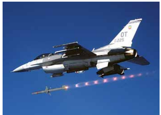
Air-to-ground munition: AGM-88 high-speed anti-radiation missile being fired from F-16C Fighting Falcon
