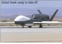
costs about US \$10 million and is powered by an Allison Rolls-Royce AE3007H turbofan engine; it carries a payload of 900 kilograms (2,000 pounds).
