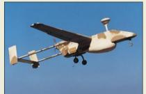
major subsystems on a manned aircraft. The Rustam, a 1.1 ton UAV, is being built to remain aloft for more than 24 hours with a range of up to 300 kilometres and a maximum altitude of 10,000 meters.
