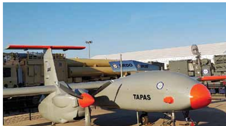
(LEFT) A MODEL OF AMCA THE ADVANCED MEDIUM COMBAT AIRCRAFT; (RIGHT) TAPAS IS A MALE UAV WITH AN OPERATING ALTITUDE OF 30,000 FT AND A RANGE OF 250 KMS.
