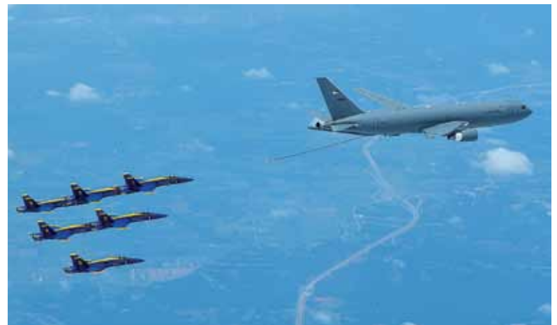
A KC-46 PEGASUS LINES UP TO REFUEL US NAVY BLUE ANGELS F/A-18 HORNET. THE KC-46 REPRESENTS THE BEGINNING OF A NEW ERA IN AIR-TO-AIR REFUELING CAPABILITY. THE MODERNISED FLY-BY-WIRE BOOM PROVIDES A LARGER AIR-REFUELING ENVELOPE.
