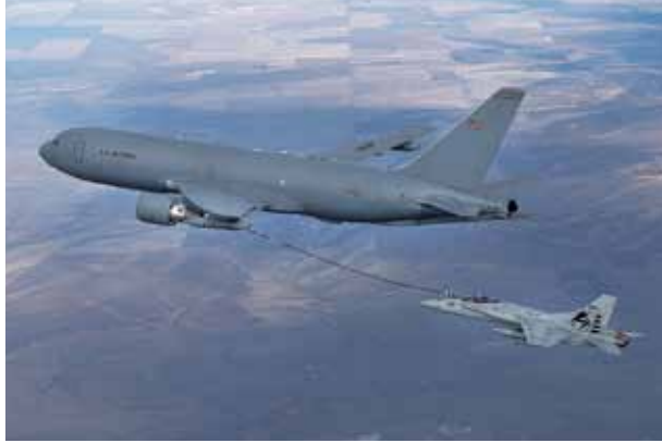
(LEFT) THE KC-46 OFFERS A PERFECT CHOICE FOR A MULTI-ROLE TANKER-TRANSPORT WHILE RETAINING THE CAPABILITY TO UNDERTAKE AERIAL REFUELLING; (RIGHT) THE KC-46 IS EQUIPPED WITH BOTH HOSE-AND-DROGUE AS WELL AS BOOM RECEPTACLE SYSTEM
