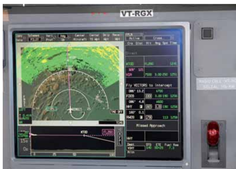
STATE-OF-THE-ART GLASS COCKPIT BY HONEYWELL IN FALCON 7X
