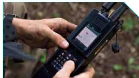
This PR4G/Fastnet soldier radio includes the latest Thales Geomux waveforms. Voice, IP data and blue force tracking data are simultaneously managed by the same device.
