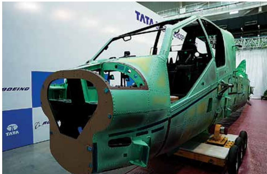
TATA BOEING AEROSPACE LIMITED (TBAL) MANUFACTURES AERO-STRUCTURES FOR BOEING'S AH-64 APACHE HELICOPTER, INCLUDING FUSELAGES
